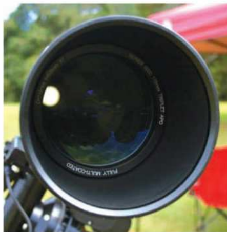
▲ The telescope's triplet objective showed reflections only under bright sunlight.
