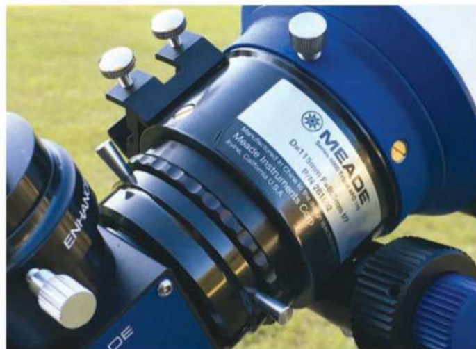
▲ Left: The beefy 3-inch focuser included with the 115 ED includes a blue anodised 10-to-1 fine-focus knob. Right: The unit's drawtube is marked in centimetres to help quickly repeat focus with your favourite eyepieces and other accessories. The 2½- to 2-inch visual back can be independently rotated by holding the large knurled ring and turning the 'captain's wheel' with aluminium pegs.
