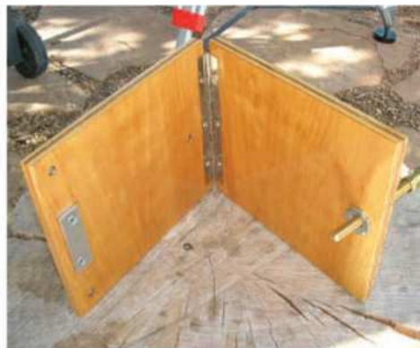
▲ The plywood version uses a piano hinge on one end and a metal plate on the other for the adjustment screw to rest on.
