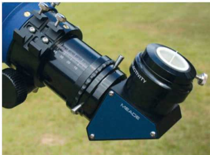
▲ Left: The beefy 3-inch focuser included with the 115 ED includes a blue anodised 10-to-1 fine-focus knob. Right: The unit's drawtube is marked in centimetres to help quickly repeat focus with your favourite eyepieces and other accessories. The 2½- to 2-inch visual back can be independently rotated by holding the large knurled ring and turning the 'captain's wheel' with aluminium pegs.
