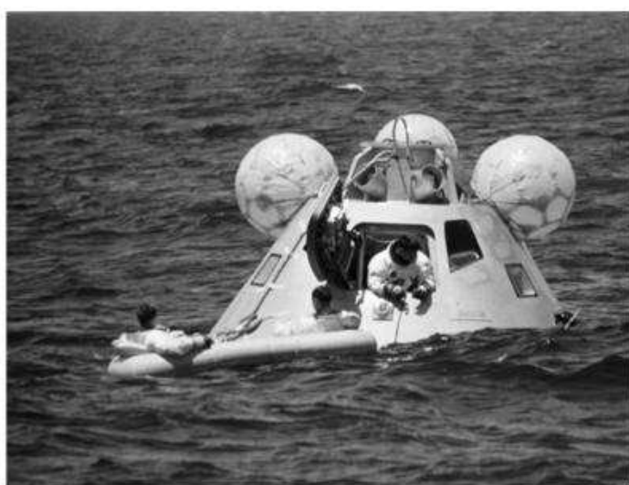
The Apollo 7 astronauts practice exiting the command module after splashdown in the Gulf of Mexico. The three balloons are meant to right the capsule after re-entry if necessary; during the actual mission, the capsule landed upside down, and the balloons worked as intended within minutes.
