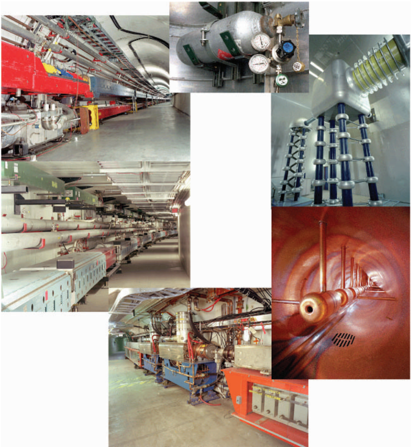
Figure 6.8 From top center, going in a clockwise direction: the hydrogen bottle from which protons are generated, the Cockcroft-Walton accelerator, the LINAC, the Booster, the Main Injector and Antiproton Recycler and finally the Tevatron and the Main Ring (the predecessor of the Main Injector). In the image containing the Tevatron, the top series of magnets is the currently-unused Main Ring, while the smaller ring of magnets is the Tevatron. (Figure courtesy of Fermilab.)
