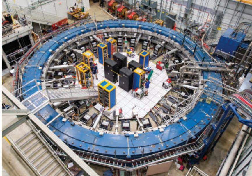
The Muon  $g-2$  experiment studies how muons wobble as they circulate at nearly the speed of light in a giant, doughnut-shaped magnet (shown). New results disagree with the standard model of particle physics, hinting at the possible existence of new particles.
